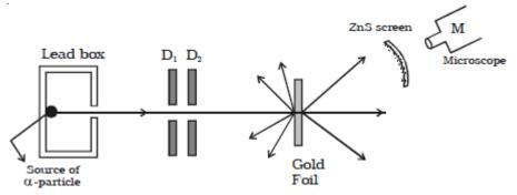
The  $\alpha$ -particles of energy 5.5MeV emitted from the source in all possible directions, but only a narrow beam emerges from the lead box. The remaining  $\alpha$ -particles are absorbed in the lead box itself. After passing through the diaphragms D1 and D2, a narrow beam of  $\alpha$ particles incident on a thin gold foil of thickness  $2.1 \times 10^{-7}$  m, are scattered through different angles.
