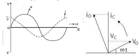
Secondly when  $\cos\omega t$  = 1, in equation  $i_C=CE_0\omega\cos\omega t$  the current in circuit is maximum
