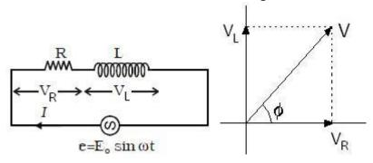
Suppose in phasor diagram, current is taken along positive direction. The  $V_R$  is also along positive x-direction as there is no phase difference between  $i_R$  and  $V_R$ . While  $V_L$  will be along y direction as we know that current lags behind the voltage by  $90^{\circ}$  So we can write
