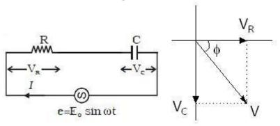
Suppose in phasor diagram current is taken along positive x-direction. Then  $V_R$  is along positive x-direction but  $V_C$  is along negative y-direction as current leads the potential by phase  $90^{\circ}$  so we can write
