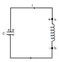
The moment the circuit is completed, the charge on the capacitor starts decreasing, giving rise to current in the circuit. Let q and i be the charge and current in the circuit at time t. Since di/dt is positive, the induced emf in L will have polarity as shown, i.e.,  $v_b < v_a$ . According to Kirchhoff's loop rule,
