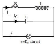
Let the instantaneous value of emf applied be V and the corresponding current is I,  $I_L$  and  $I_C$ . Then
