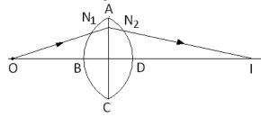
Lens shown in diagram have two curved surfaces. Surface ABC ( $N_1$ ) have radius of curvature  $R_1$ . Another surface ADC ( $N_2$ ) have radius of curvature  $R_2$ . Image formed by Surface  $N_1$  acts as an object for surface  $N_2$  and final image is formed at I
