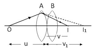
Consider two lenses A and B of focal length  $f_1$  and  $f_2$  placed in contact with each other. Let the object be placed at a point O beyond the focus of the first lens A.
