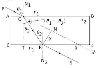
As shown in figure light ray undergoes refraction twice, once at top (AB) and then from bottom (CD) surfaces of given homogeneous medium.
