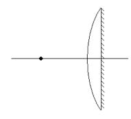
Q) The plane surface of a plano-convex lens of focal length 60 cm is silvered . A point object is placed at a distance 20cm from the lens. Find the position and nature of the final image formed
