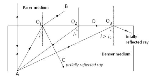
When light travels from optically denser medium to rarer medium at the interface, it is partly reflected back into same medium and partly refracted to the second medium. This reflection is called the *internal reflection*.
