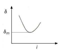
From the graph  $\delta$  vs i we can find that for every angle of deviation there are two values of angle of incidence. It means that vale of i and e are interchangeable. Except i=e . At i =e the angle of deviation is minimum denoted by  $\delta_m$  or  $D_m$ , at angle of minimum deviation ray inside the prism becomes parallel.
