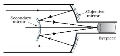
Telescopes with mirror objectives are called *reflecting* telescopes.
