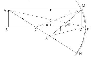
As shown in figure AB is object while A'B' is image of the object . AM and AN are two incident rays emitted from point A. Let F be focal point and FD = f focal length
