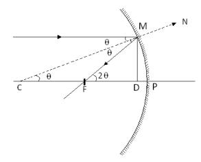
Let P the pole of concave mirror, F be focal point and C be the centre of curvature.
