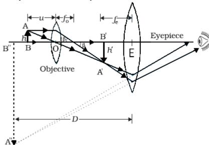
A simple microscope has a limited maximum magnification ( $\leq$  9) for realistic focal lengths. For much larger magnifications, one uses two lenses, one compounding the effect of the other. This is known as a *compound microscope*.
