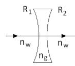
Q) Calculate the focal length of a concave lens in water (Refractive index = 4/3) if the surface have radii equal to 40cm and 30 cm (refractive index of glass = 1.5)
