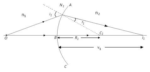
$$\frac{n_2}{v_1} - \frac{n_1}{u} = \frac{n_2 - n_1}{R_1} \dots eq(1)$$
