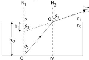
$n_i$  is the refractive index of observer medium,  $n_o$  is the refractive index of object medium.  $h_o$  is the real depth and  $h_i$  is virtual depth.
