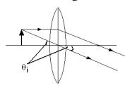
We now find the angle subtended at the eye by the image when the object is at u. From the relations  $m = \frac{h'}{h} = \frac{v}{v}$
