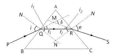
PQ is incident ray and angle made by PQ with normal is i. QR is refracted ray at surface BA and angle of refraction is  $r_1$
