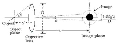
Let the diameter of lens be D and its focal length be f. As object distance is usually kept greater than that of f. Let the image distance be v. the angular width of central maximum due to the effect of diffraction is ,
