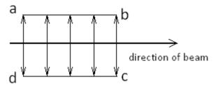
"The plane containing the direction of the beam and the direction of oscillation of E vectors is called the plane of oscillation . In figure abcd is the plane of oscillation
