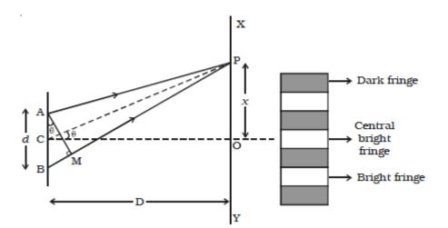
Draw AM perpendicular to BP The path difference  $\delta = BP - AP AP = MP$   $\therefore \delta = BP - AP = BP - MP = BM$ In right angled  $\Delta ABM$ ,  $BM = d \sin \theta$ If  $\theta$  is small,  $\sin \theta = \theta$   $\therefore$  The path difference  $\delta = \theta.d$ In right angled triangle COP,
