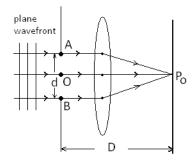
Consider a plane wavefront arrive at a plane of slit, according to Huyen's principle all the point on the slit like AOB acts as secondary source having the same phase and produce secondary waves.
