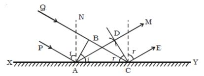
Therefore CD is the reflected plane wavefront and AD is the reflected ray.
