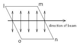
"A plane perpendicular to the plane of oscillation and passing through the beam of light is called the plane of polarization"
