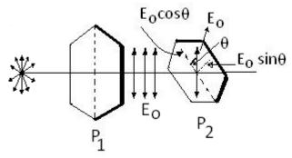
Thus, only  $E_0\cos\theta$  components will emerge out of plate  $P_{2'}$  while perpendicular components are absorbed. Since intensity is proportional to the square of amplitude, intensity of light incident on plate  $P_2$  is
