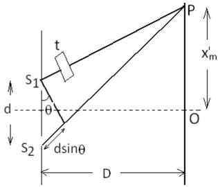
Path difference before placing slab =  $S_2P - S_1P = r_2 - r_1 = \delta$ On placing slab path length of thickness t effective path length  $S_1P = (r_1 - t) + t\mu$ Thus effective path difference after placing slab  $\delta' = r_2 - [(r_1 - t) + t\mu]$  $\therefore \delta' = (r_2 - r_1) + t(\mu - 1)$
