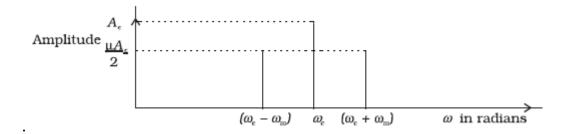
Amplitude of USB and LSB is μA<sub>c</sub>/2
