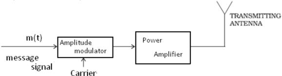
Modulated signals cannot be transmitted as such. The modulator is followed by a power amplifier which provides the necessary power and then modulated signals is forwarded to an antenna of appropriate size for radiation as shown in figure
