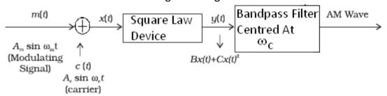
Here the modulating signal  $A_m \sin \omega_m t$  is added to the carrier signal  $Ac \sin \omega_c t$  to produce the signal x(t). This signal  $x(t) = A_m \sin \omega_m t + Ac \sin \omega_c t$  is passed through a square law device which is a non-linear device which produces an output
