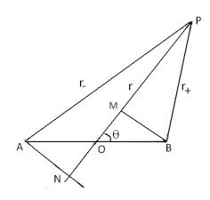
Let a dipole consisting of equal and opposite charge q separated by a distance 2a. Let zero of coordinate system is at centre of the dipole as shown in figure. Let p be any point in x-y plane. Let PO = r. AP =  $r_-$  BP =  $r_+$ . Let r makes angle of  $\theta$  with the axis of dipole.
