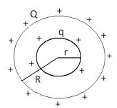
Suppose there is a positive charge Q, on an insulated conducting spherical shell of radius R, as shown in figure. At the centre of this shell, there is a conducting sphere of radius r (r<R), having a charge q.
