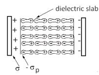
Consider a dielectric inserted between the plates of capacitor, the dielectric is polarized by the electric field, the effect is equivalent to two charged sheets with surface charge densities  $\sigma_P$  and  $-\sigma_P$ . The electric field in the dielectric will be
