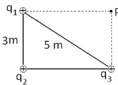
$q_3$  = 3 $\mu$ C are fixed at position shown in figure (a) What is the potential at point P at the corner of the rectangle? (b) How much work would be needed to bring a charge  $q_4$  = 2.5  $\mu$ C from infinity to place it at P
