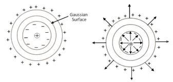
Consider a +q<sub>0</sub> suspended in a cavity in a conductor. Consider. Consider a Gaussian surface just outside the cavity and inside the conductor  $\vec{E}$  =0 on this Gaussian surface as it is inside the conductor form Gauss's law
