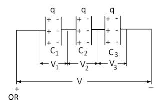
Capacitor are said to be connected in series if charge on each individual capacitor is same. In this situation
