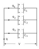
When capacitors are connected in parallel, the potential difference V across each is same and the charge on  $C_1$ ,  $C_2$  and  $C_3$  is different i.e  $q_1$ ,  $q_2$  and  $q_3$
