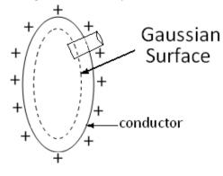
Consider a Gaussian surface of a pill-box of extremely small length and extremely small cross-section ds. A fraction of it is inside the surface and the remaining part is outside the surface . The total charge enclosed by this pill-box is  $q=\sigma ds$ , where  $\sigma=surface$  charge density of the charge on the conductor. At every point on the surface of the conductor  $\vec{E}$  is perpendicular to the local surface element. Hence it is parallel to the
