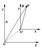
Two frame of reference A and B as shown in figure moving with uniform velocity with respect to each other. Such frame of references are called inertial frame of reference. Suppose two observers, one in from A and one from B study the motion of particle P.
