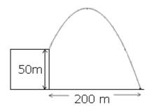
Let v be the velocity of projectile Velocity along x-axis,  $V_x = v\cos\theta$ Let t be the time of flight Displacement along x-axis X, 200= (vcos $\theta$ ) t
