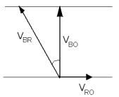
Suppose the river is flowing in positive X direction as shown in figure . To reach to a place in the perpendicular direction on the other bank, the boat has to move in the direction making angle  $\theta$  with Y direction as shown in figure. This angle should be such that the velocity of the boat relative to the opposite bank is in the direction perpendicular to the bank . Let  $V_{\text{BR}}\,$  = Velocity of boat with respect to river
