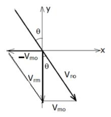
From figure  $\sin\theta = V_{mo}/V_{rm} = 3/V_{rm}$
