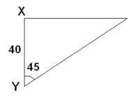
Let velocity of interceptor speed be V . Now components of velocity along North direction is Vcos45 and along East direction is Vsin45
