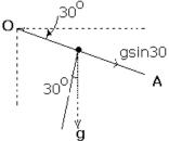
$v^2 = u^2 + 2as$  $v^2 = 0^2 + 2 \times 4.9 \times 2.45 \Rightarrow v = 4.9 m/s$ Now horizontal component of velocity which causes horizontal displacement.
