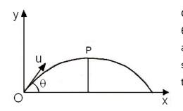
Consider a particle projected with a velocity u of an angle  $\theta$  with the horizontal earth's surface. If the earth did not attract a particle to itself, the particle would describe a straight line, on account of attraction of earth, however, the particle describes a curve path
