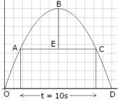
Time taken by projectile to travel from point B to C is 5 sec.
