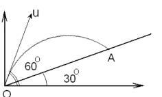
a = 30° and the angle of barrel to the horizontal is  $\beta$  = 60°. The initial velocity of shell is 21 m/s. Find the distance from gun to the point at which the shell falls
