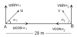
If both the particles have same initial vertical velocity v then only particles will collide so that for collision both particles must be at same height
