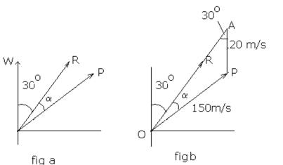
In fig(a) Vector W represents direction of velocity of wind. Vector P represents direction of plane and vector R represents position where plane has to go.
