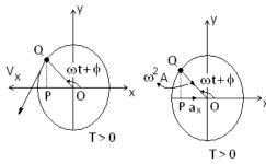
In figure shown Q is a point moving on a circle of radius A with constant angular speed  $\omega$  (in rad/sec). P is the perpendicular projection of Q on the horizontal diameter, along the x-axis.
