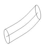
In a fluid having a steady flow, if we select a finite number of streamlines to form a bundle
