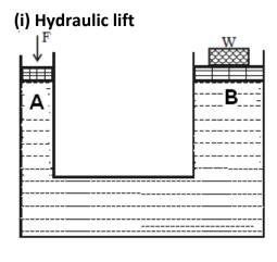
An important application of Pascal's law is the hydraulic lift used to lift heavy objects. A schematic diagram of a hydraulic lift is shown in the Fig.. It consists of a liquid container which has pistons fitted into the small and large opening cylinders. If  $a_1$  and  $a_2$  are the areas of the pistons A and B respectively, F is the force applied on A and W is the load on B, then
