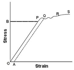
(i) In the figure the region OP is linear. Within a normal stress, strain is proportional to the applied stress. This is
