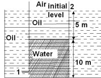
tank of same oil. Water flows through the hole. What is the velocity of the flow initially? When the flow stops, what would be the position of the oil-water interface in the tank? The ratio of the cross-section area tank to the that of hole is 50, determine the time at which the flow stops, density of oil =  $800 \text{ kg/m}^3$
