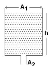
Let  $v_1$  and  $v_2$  be the speeds of the liquid at  $A_1$  and  $A_2$ . As both the cross sections are opened to the atmosphere, the pressure there equals to atmospheric pressure  $P_o$ . If the height of the free surface above the hole is  $h_1$
