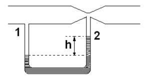
This is a device based on Bernoulli's principle used for measuring the flow of a liquid in pipes. A liquid of density  $\rho$  flows through a pipe of crosssectional area A. Let the constricted part of the cross-sectional area be 'a'. A manometer tube with a liquid say mercury having a density  $\rho_0$  is attached to the tube as shown in figure
