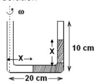
when tube is rotated liquid will experience a centrifugal force thus water moves up in second arm of the U tube.
