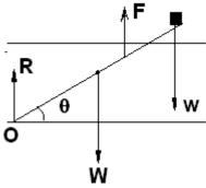
Moment of force due to weight of rod about point  $O=Wg(L/2)cos\theta$ Moment of force due to additional weight about point  $O=wLcos\theta$ Moment of force due to Buoyant force(F) about point  $O=F(I/2)cos\theta$ Here l is the length of rod immersed in water =5m And L is total length of rod
