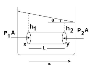
When a vessel filled with liquid accelerates horizontally. We observe its free surface inclined at some angle with horizontal. To find angle  $\theta$  made by free surface with horizontal, consider a horizontal liquid column including two points x and y at the depth of  $h_1$  and  $h_2$  from the inclined free surface of liquid as shown in figure
