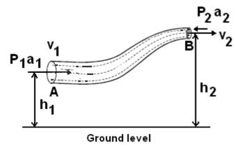
Consider streamline flow of a liquid of density  $\rho$  through a pipe AB of varying cross section.
