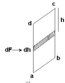
The point of application of the force on the wall can be calculated by equating the moment of resultant force about any line, say dc to the moment of distributioed force about the same line dc
