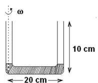
open to a pressure  $1.01\times10^3$  N/m<sup>2</sup>. Water is poured into the tube such that liquid just fills horizontal part of the tube is then rotated about a vertical axis passing through the other vertical arm with angular velocity  $\omega$ . If length of water in sealed tube rises to 5cm, calculate  $\omega$ . Take density of water =  $10^3$  kg/m<sup>3</sup> and g = 10 m/s<sup>2</sup>. Assume temperature to be constant.
