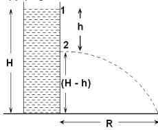
$$P_1 + \rho g h_1 + \frac{1}{2} \rho v_1^2 = P_2 + \rho g h_2 + \frac{1}{2} \rho v_2^2$$
