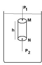
When gravity is taken into account, Pascal's law is to be modified. Consider a cylindrical liquid column of height h and density  $\rho$  in a vessel as shown in the Fig.
