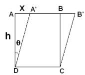
In figure a body with square cross section is shown a tangential force acts on the top surface AB causes shift of Surface by 'X' units shown as surface A'B' ,thus side DA' now mates an angle of  $\theta$  with original side DA of height h
