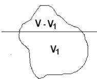
Let a solid of volume V and density  $\rho$  floats in liquid of density  $\rho_0$ . Volume V<sub>1</sub> of the body is immersed inside the liquid
