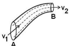
∴ Volume of liquid entering per second at  $A = a_1v_1$ .
