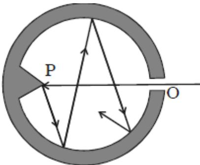
Fery's black body consists of a double walled hollow sphere having a small opening O on one side and a conical projection P just opposite to it. Its inner surface is coated with lamp black. Any radiation entering the body through the opening O suffers multiple reflections at its inner wall and about 97% of it is absorbed by lamp black at each reflection. Therefore, after a few reflections almost
