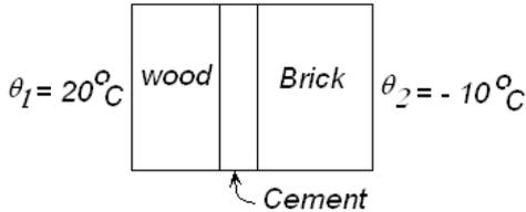
The thermal resistance of wood, the cement and the brick layers are
