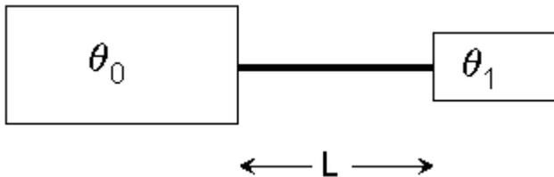
containing a mass  $m$  of water at an initial temperature  $\theta_1 (<\theta_0)$ . A metal rod of length  $L$ , area of cross-section  $A$  and thermal conductivity  $K$  connects the two vessels.
